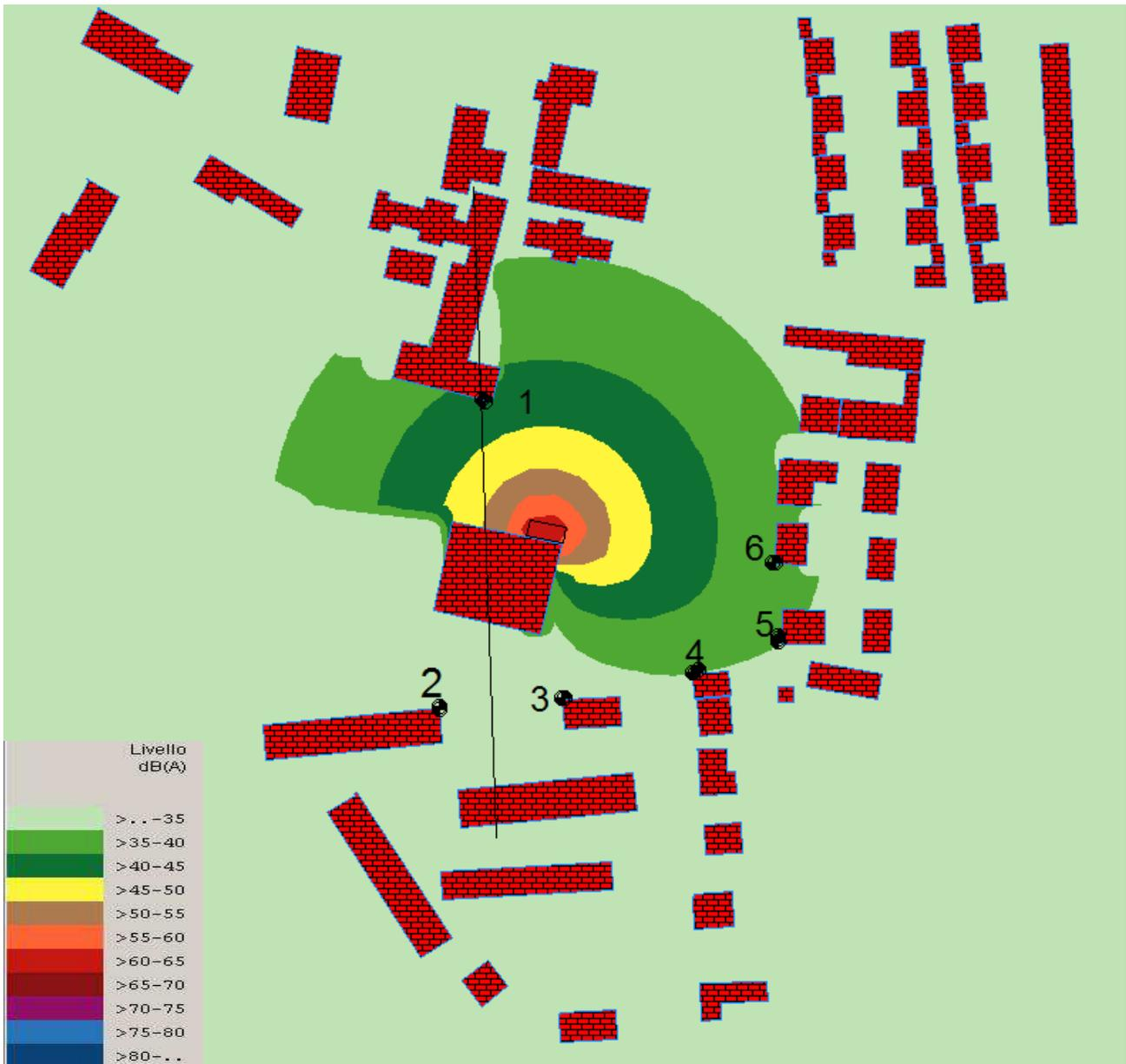
**EMISSIONE NOTTURNA IMPIANTI TECNICI CON BARRIERA IN COPERTURA**
